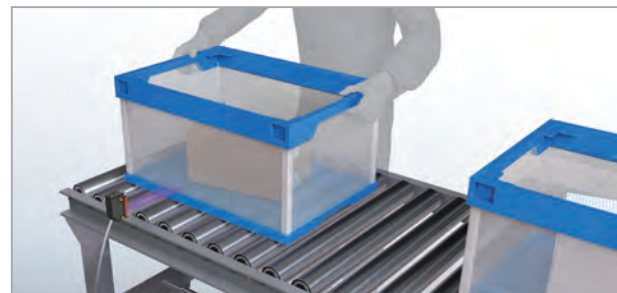
Inspection and carry lines Reliable detection of the target only, not the worker.
