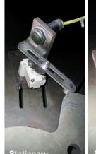
Shock: Approx. 50G conditions | Shock application speed: 240 cycles/min
