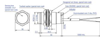
Note: When the sensor is flush-mounted in metal, be sure to mount it so that the top of the sensing face projects 2 to 2.5 mm from the metal surface. M12 type=2 mm M18 and M30 type=2.5 mm
