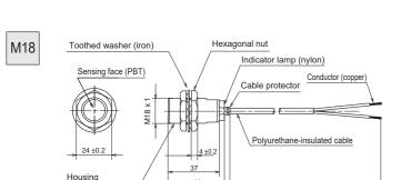
Insulated cable (oil-resistant, 0.5 mm<sup>2</sup>, 20/0.18 dia., 2-core), dia. 5.7
