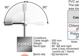
PVC and PUR cables are tested according to the conditions shown to the left. The table below shows the number of bends before the cable's electrical connection
