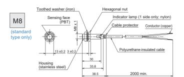
Insulated cable (oil-resistant, 0.3 mm<sup>2</sup>, 27/0.12 dia., 2-core), dia. 4.1 Cap color: blue
