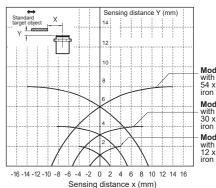
Model FL7M-8\_6A\_ with standard 54 x 54 x 1 mm iron target object Model FL7M-4\_6A\_ with standard 30 x 30 x 1 mm iron target object Model FL7M-2\_6A\_ with standard 12 x 12 x 1 mm iron target object
