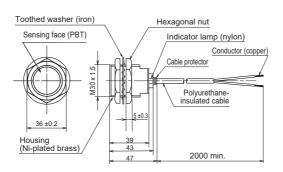
Insulated cable (oil-resistant, 0.5 mm², 20/0.18 dia., 2-core), dia. 5.7
