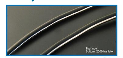
In contrast, polyurethane (PUR) cable retains almost the same appearance and performance.
