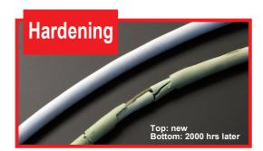
As seen above, chloromethane (PVC) cables become severely deteriorated.
