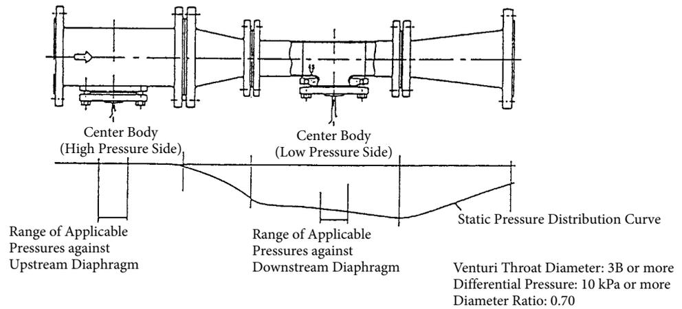
Figure 3-10. Venturi Tube Assembly
