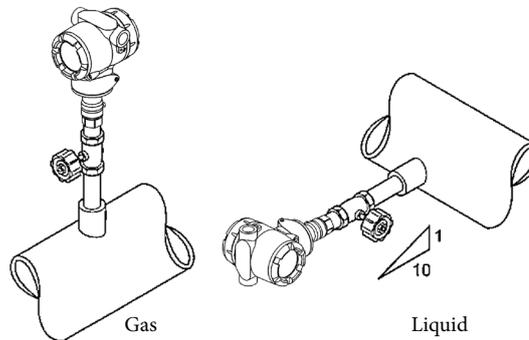
Figure 2-32. Direct Mounting Instrumentation Example
