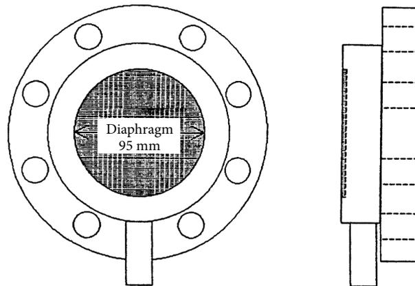
Figure 2-10. Full View of Pressure Receiver
