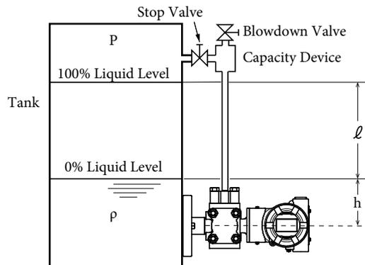
Figure 2-9. Liquid Level Measurement (by GTX\_F) of Sealed Tank with Gas Seal (Dry Leg) Connecting Pipe
