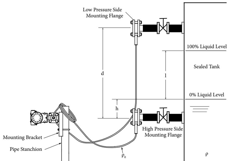
Figure 3-25. When Tank is Sealed
