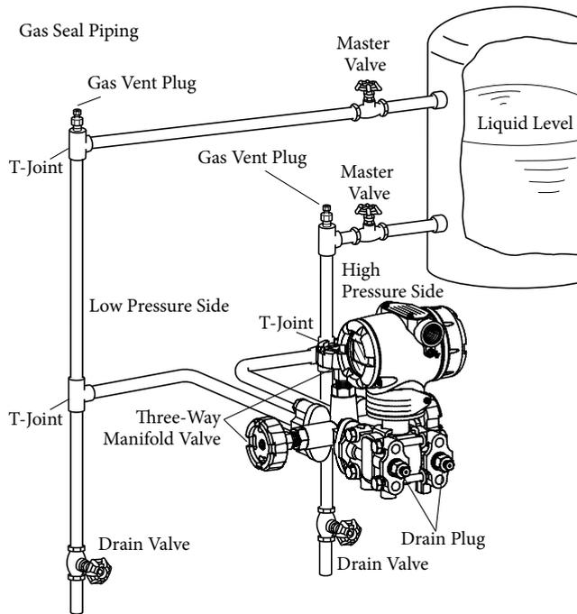
Figure 2-47. Closed Tank, Dry Leg Piping Example
