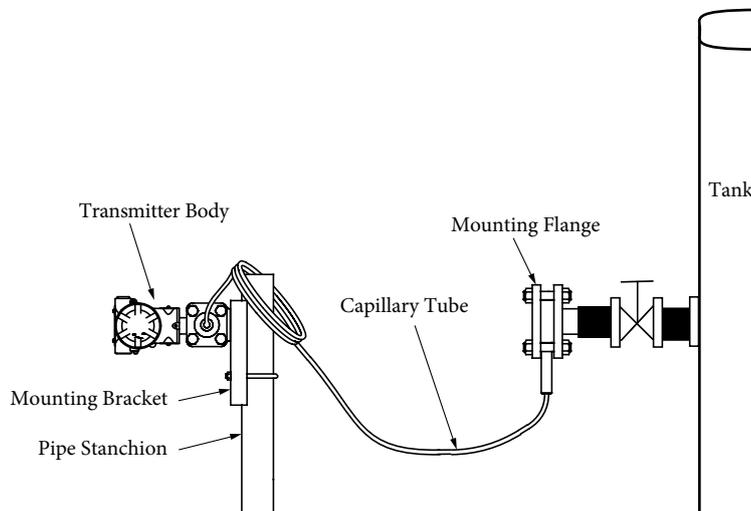
Figure 2-13. Example of Mounting on an Open Tank
