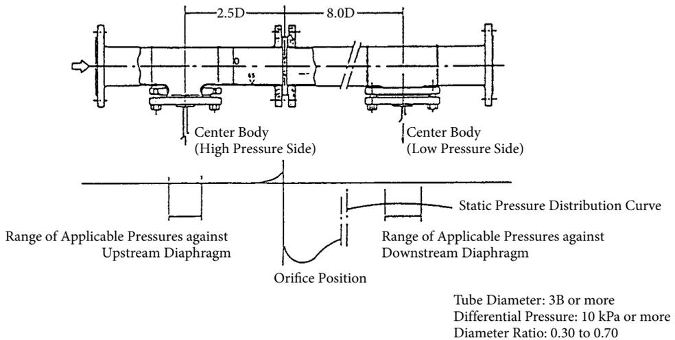
Figure 3-9. Orifice Plate Assembly
