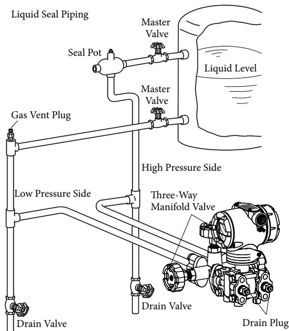
Figure 2-48. Closed Tank, Wet Leg Piping Example
