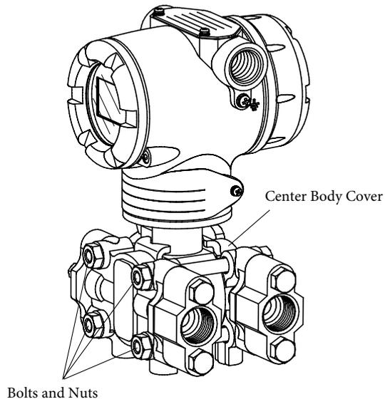
Figure 6-2. Fastening Bolt for the Center Body Cover
