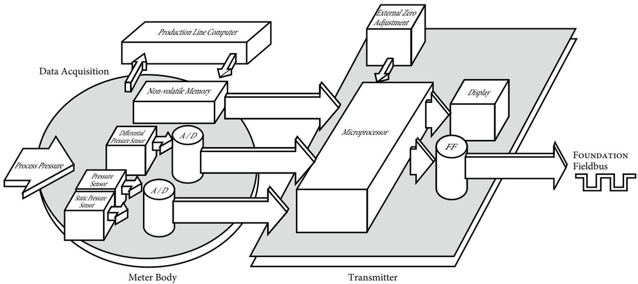
Figure 1-1. Block Diagram of this Device
