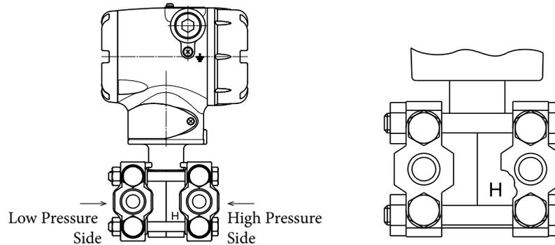
Figure 2-38. Mark on High Pressure Side of Center Body
