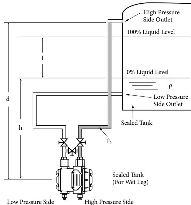
Figure 3-22. In the Case of Sealed Tank (For Wet Leg)
