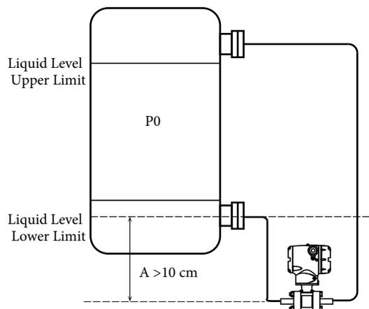
Figure 2-5. Example of Sealed Tank Level Measurement
