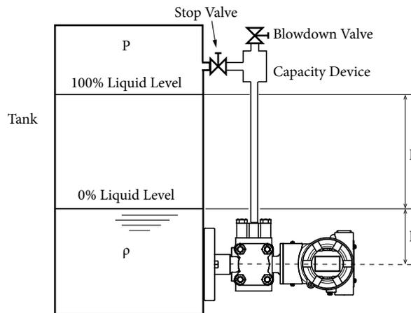
Figure 3-19. When Tank is Open (Dry Leg)
