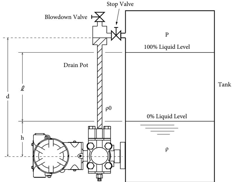
Figure 3-23. In the Case of Sealed Tank (for wet leg)
