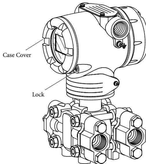
Figure 6-1. Locking the Equipment (Model GTX\_\_D)
