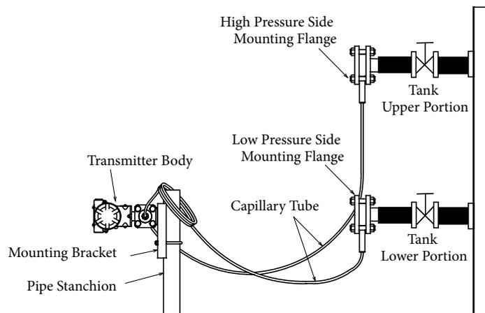
Figure 3-13. Adjusting the Actual Level during Liquid Level Measurement
