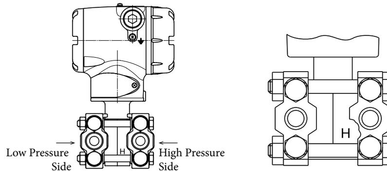
Figure 2-42. Mark on High Pressure Side of Center Body
