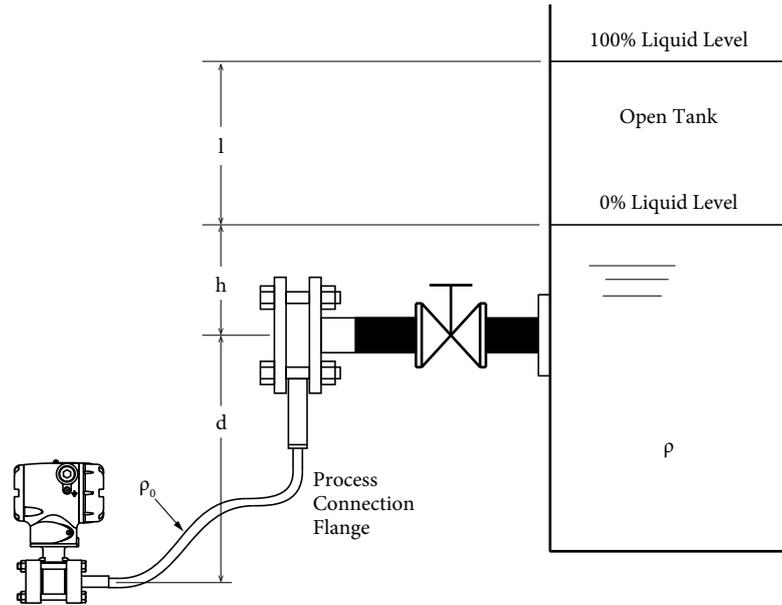
Figure 3-21. When Tank is Open
