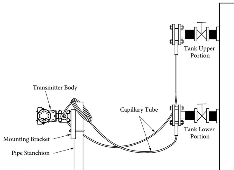
Figure 2-12. Example of Mounting on a Sealed Tank
