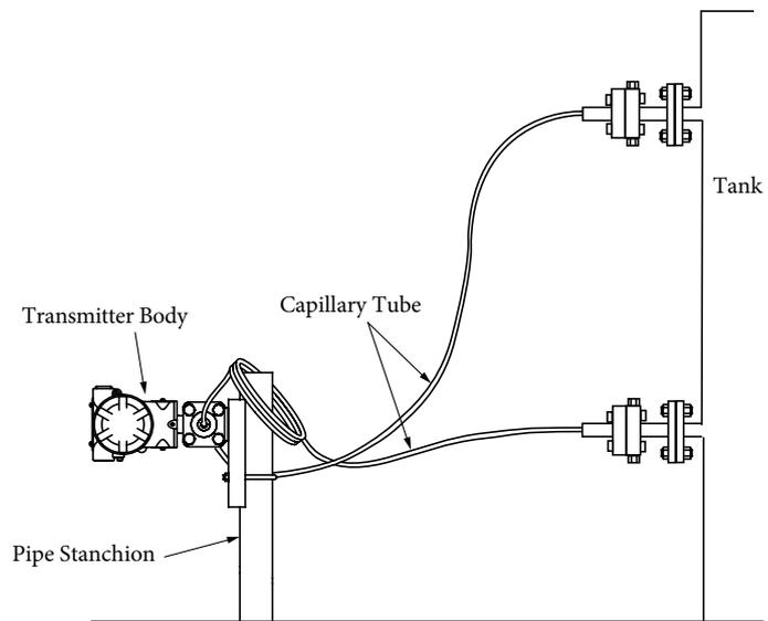
Figure 2-31. Tank Level Instrumentation Example
