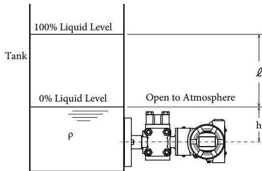
Figure 2-8. Measuring the Liquid Level of Sealed Tank (GTX\_F)
