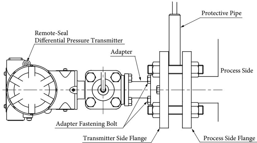
Figure 2-22. Adapter Assembly Diagram (for GTX\_\_R)
