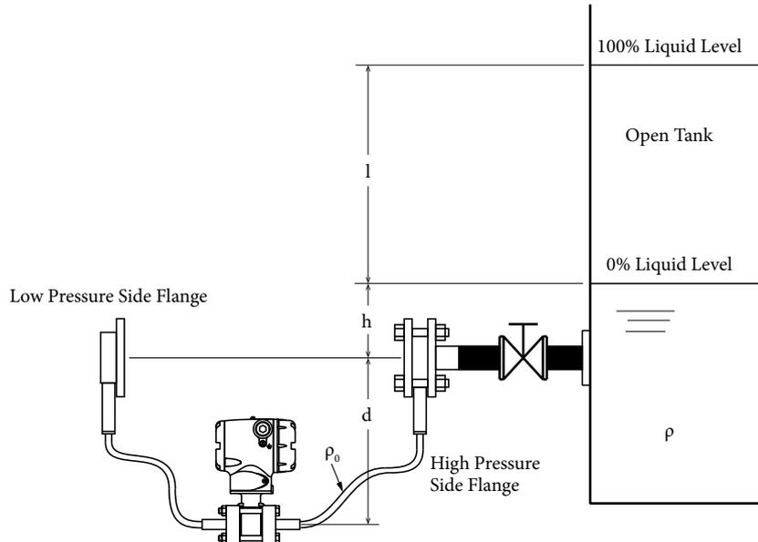
Figure 3-20. When Tank is Open
