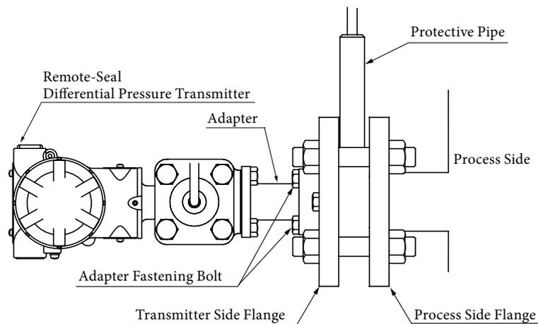
Figure 2-27. Mounting the Transmitter Flange
