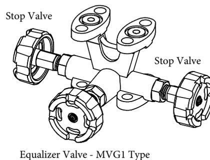
Figure 2-36. Three-Way Manifold Valve
