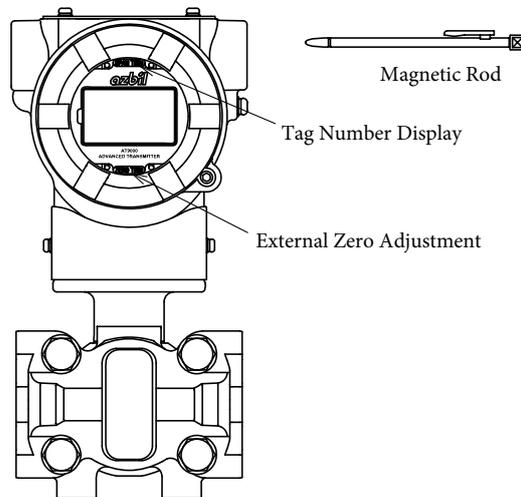
Figure 3-14. External Zero Adjustment
