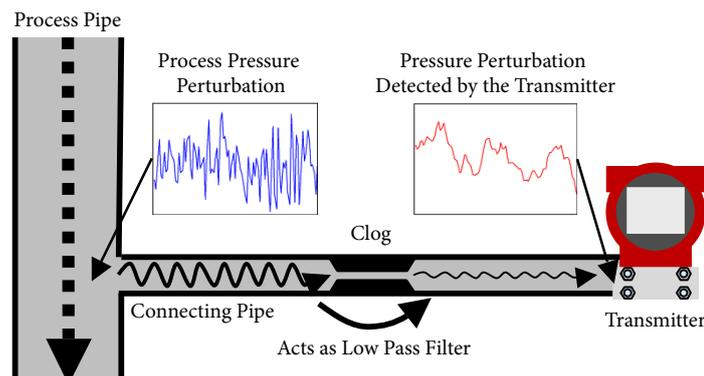
The pressure frequency index is an index of the frequency of volatile movements of the pressure perturbation, and reflects the perturbation frequency. Therefore, the clogging of the connecting pipe acts as a low pass filter; if the high frequency components of the perturbation can be minimized, then the index value will also decrease. With this system, the clogging of connecting pipe is diagnosed according to the pressure frequency index.
