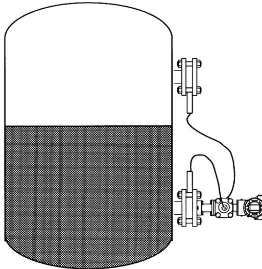
Figure 2-28. Mounting the Process-Side Flange (Example 2)
