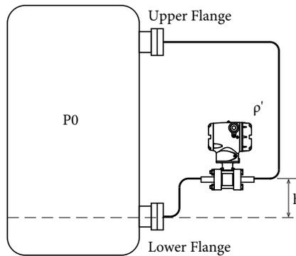
Figure 2-6. Installation Position on the Sealed Tank
