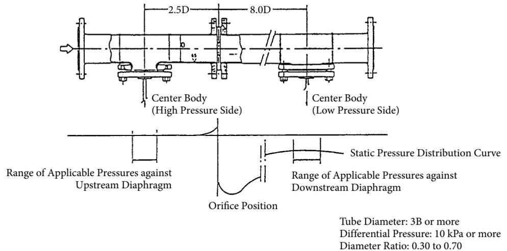
Figure 3-6. Orifice Plate Assembly
