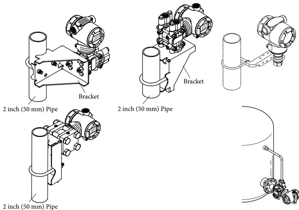
Figure 2-1. Typical Bracket Mounted and Flange Mounted Installations
