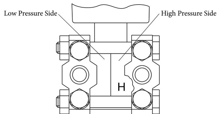
Figure 2-45. Mark on High Pressure Side of Center Body
