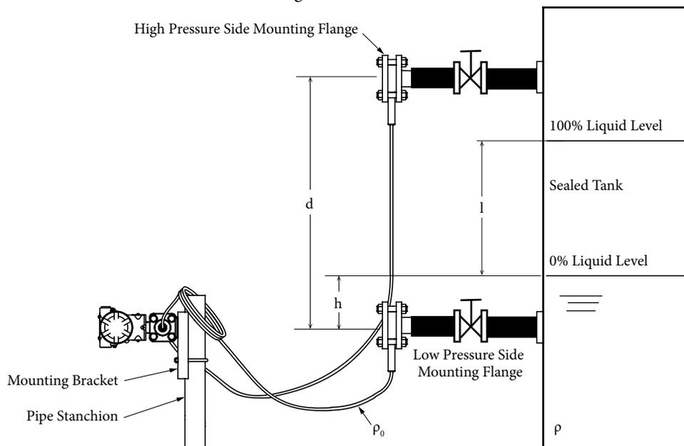
Figure 3-24. When Tank is Sealed
