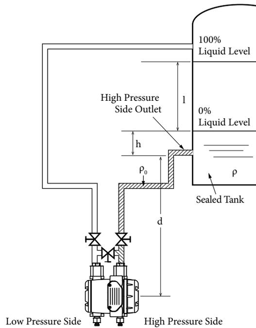
Figure 3-16. When Tank is Open (Dry Leg)
