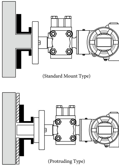
Figure 2-7. Tank Connection Diagram
