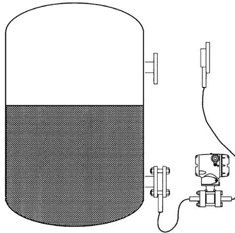
Figure 2-26. Mounting the Process-Side Flange (Example 1)
