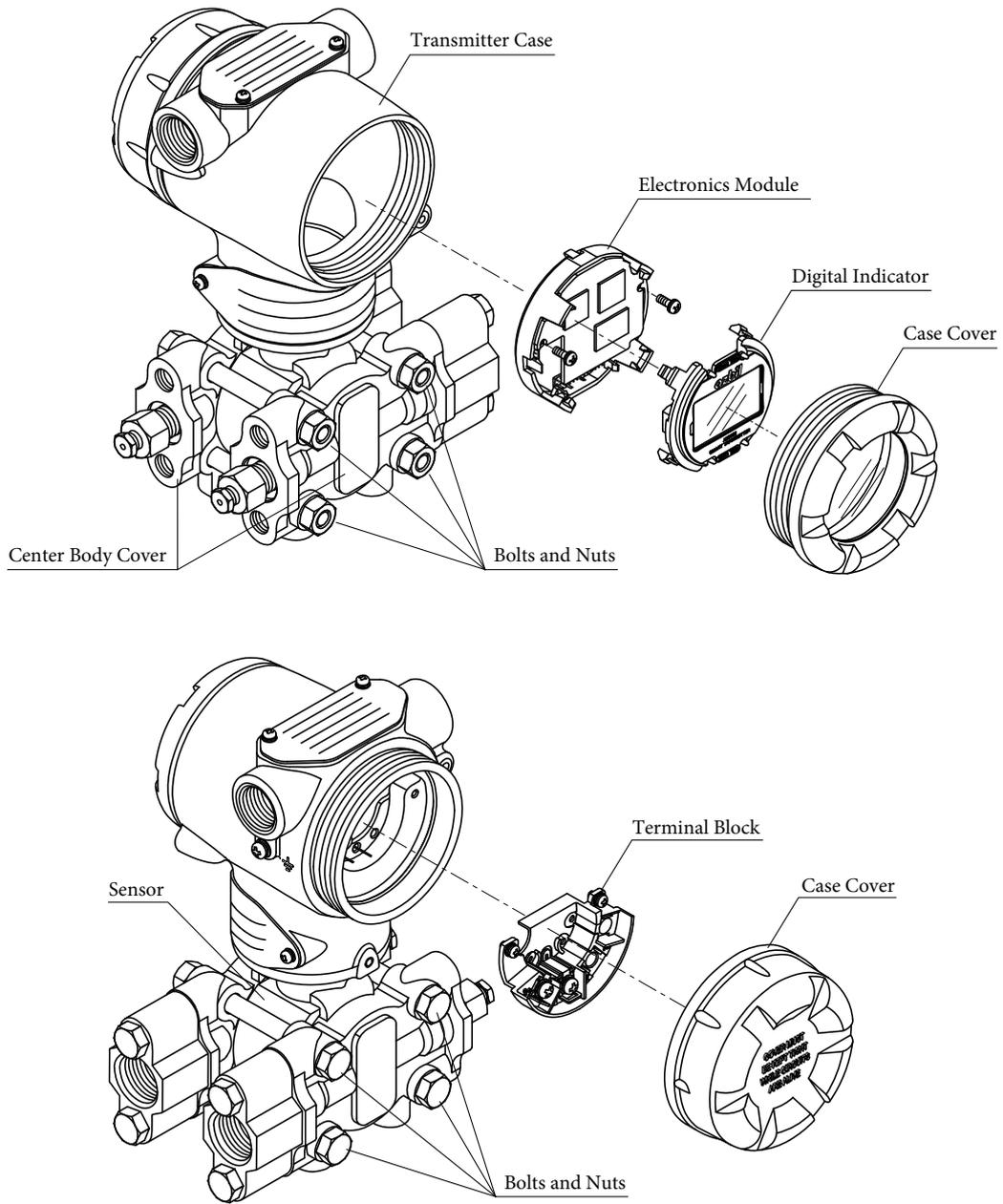
Figure 1-2. Transmitter Structure
