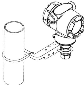
Figure 2-35. Example of Installation on 2 inch Pipe with Mounting Bracket
