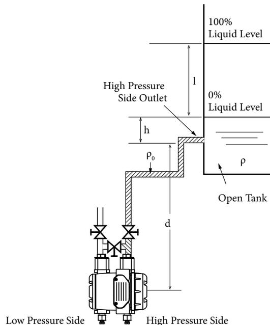
Figure 3-15. When Tank is Open
