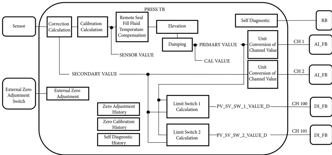
Figure 4-1. PRESS TB Function Block Diagram
