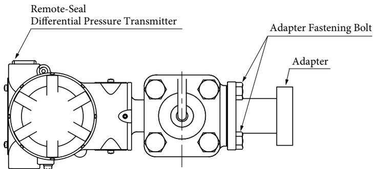
Figure 2-25. Transmitter Adapter Mount
