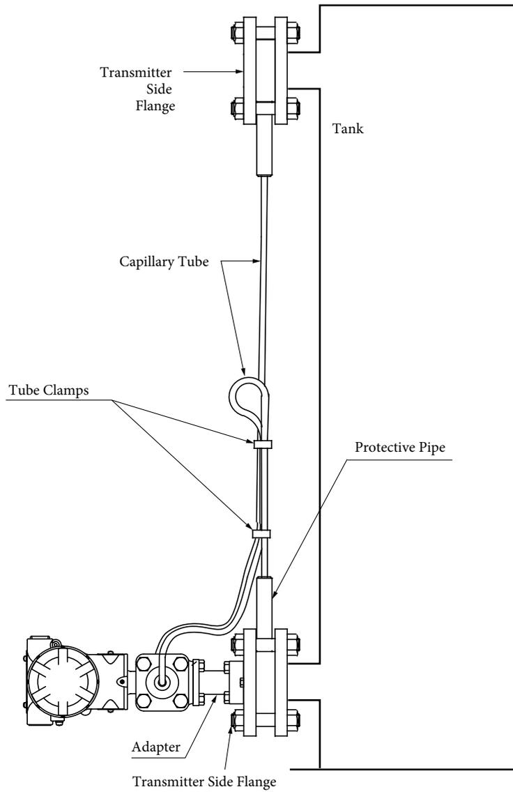
Figure 2-20. Direct-Mounting Installation Example
