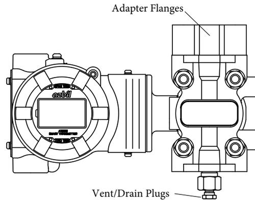
Figure 2-50. Changing the Vertical Position of the Process Connection Port
