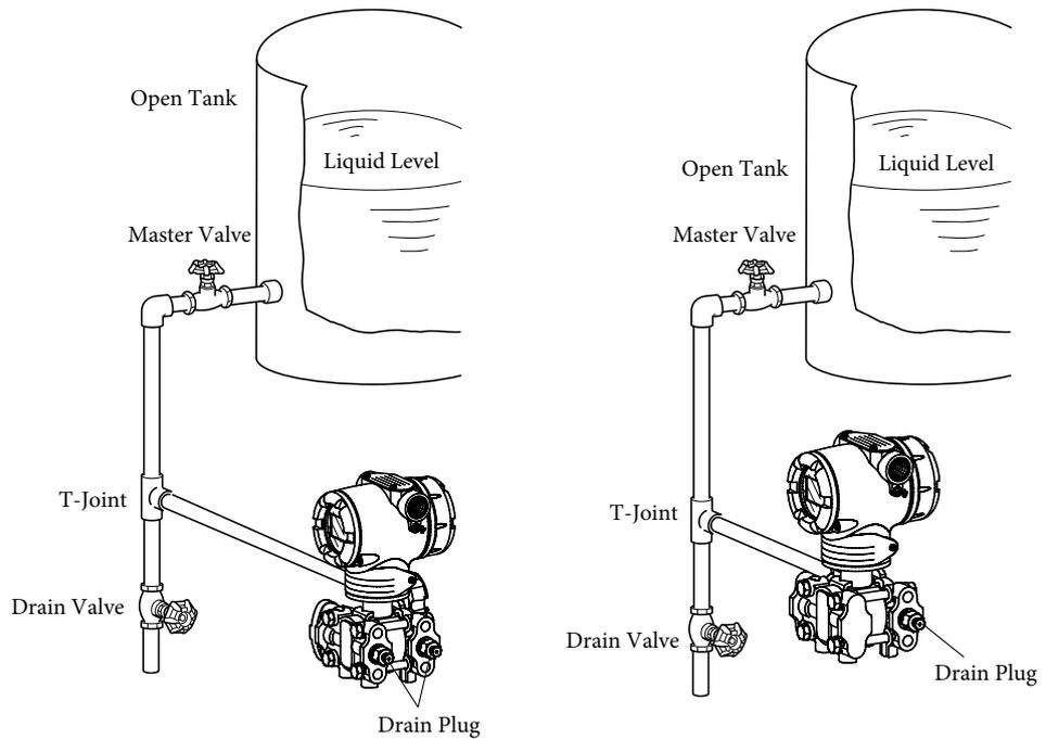
Figure 2-46. Open Tank Piping Example
