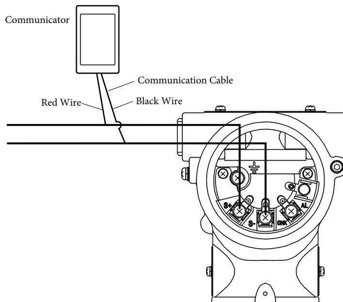
Figure 3-1. Connection with Communicator
