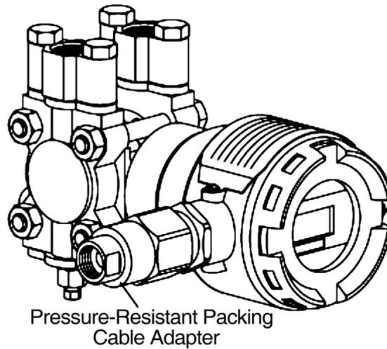
Figure 2-49. Pressure-Resistant Packing Cable Gland
