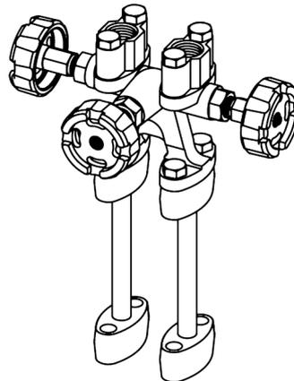
Figure 2-32. Extension Pipes
