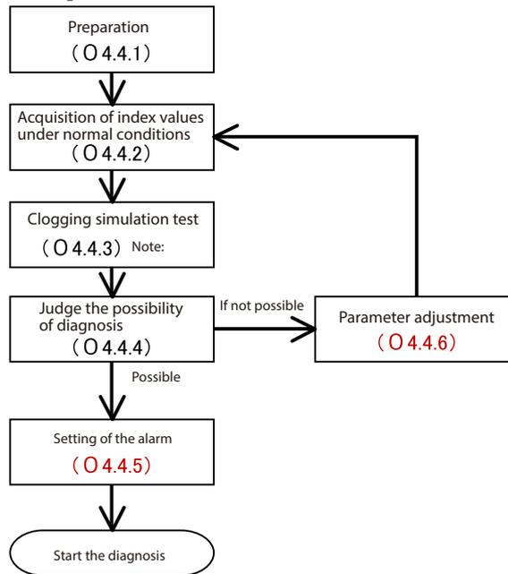
Preparation (see section A4-4-1): Initialize the parameters in preparation for obtaining the index values.
