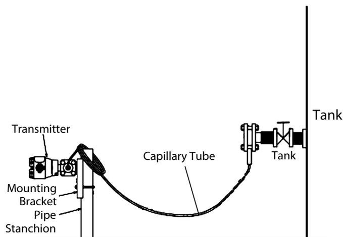
Figure 2-9. Attachment to Open Tank (JTH/JTS Model)
