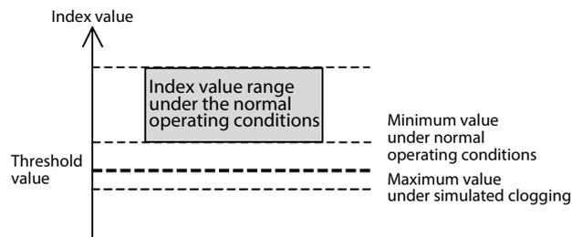
After determining the threshold value, follow the steps below to set the alarm and start the diagnosis.
