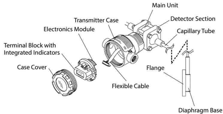
Figure 1-4. Structure of JTE and JTH Models
