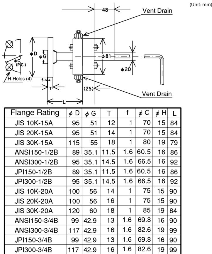
Figure 2-25. 1/2B Remote Adapter Assembly Diagram and Dimensions
