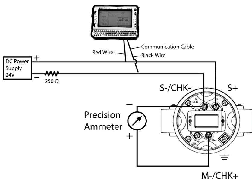
Figure 4-4. Wiring
