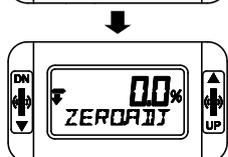
When zero point adjustment is complete, remove the magnetic stick.
