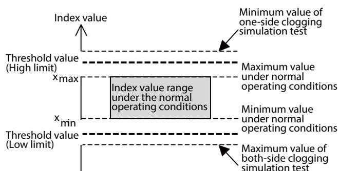
After determining the threshold value, follow the steps below to set the alarm and start the diagnosis.
