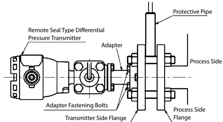
Figure 2-22. Attachment to the Transmitter Side Flange
