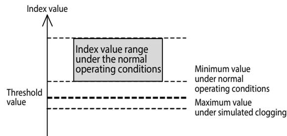
After determining the threshold value, follow the steps below to set the alarm and start the diagnosis.
