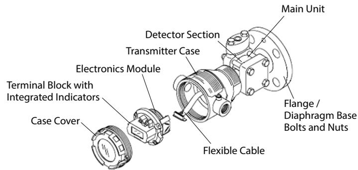
Figure 1-3. Structure of JTC Model
