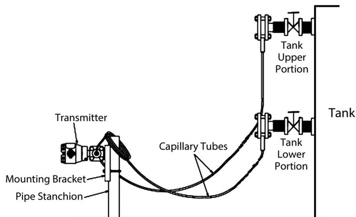
Figure 2-8. Attachment to Sealed Tank (JTE Model)
