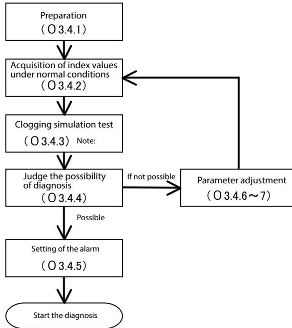
Preparation (see section A3-4-1): Initialize the parameters in preparation for obtaining the index values.
