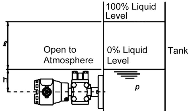
Figure 2-44. Liquid Level Measurement (Open Tank) Piping Example
