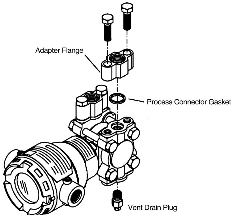
Figure 2-50. Changing Vertical Position of Process Connection Port
