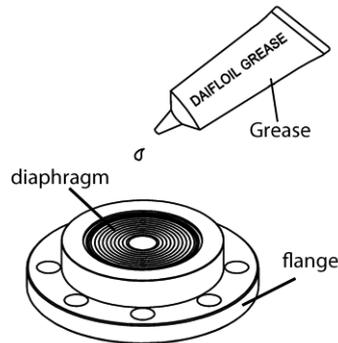
Figure 2-10. Application of Grease
