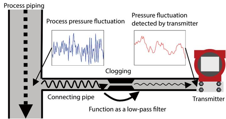
The pressure frequency index, based on the number of times the pressure rises and falls, indicates the frequency of pressure fluctuation. Clogging in the connecting pipe functions as a low-pass filter that attenuates the high-frequency components of fluctuation, thereby decreasing the index number. Because of this mechanism, clogging in the connecting pipe can be diagnosed from the pressure frequency index.
