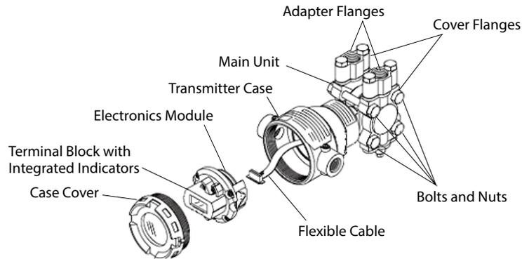
Figure 1-2. Structure of JTD Model
