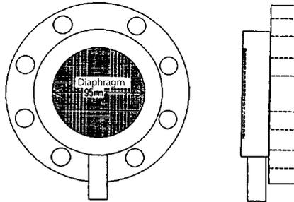
Figure 2-6. 3B Flash Mount Type Diaphragm Diameter
