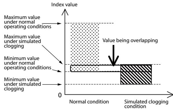
In this case, it is necessary to examine the cause of the large variation that occurs under normal conditions, and to reduce this effect. Use the following the guidelines for adjustment.
