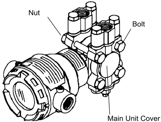
Figure 4-2. Nuts and Bolts Fastening the Main Unit Cover
