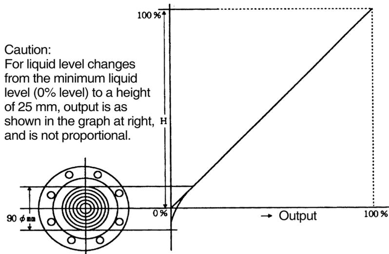
Figure 3-6. Minimum Liquid Level Characteristics
