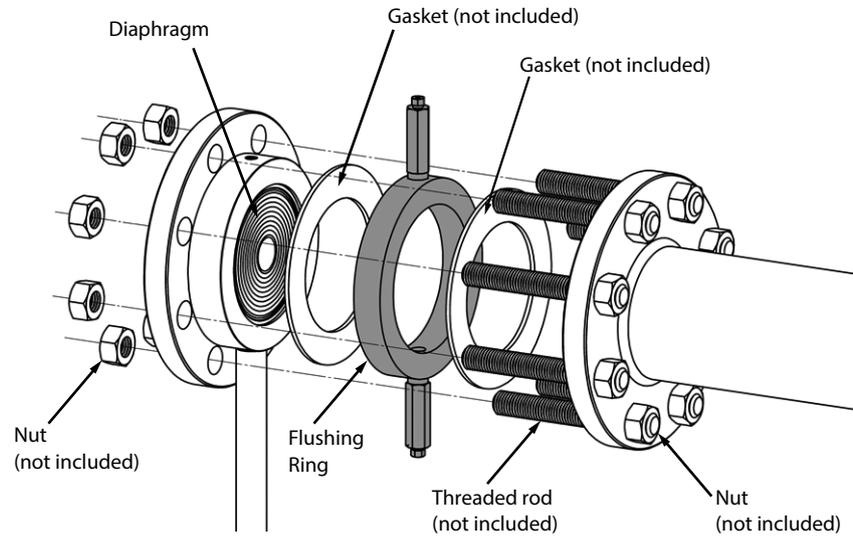
Figure 2-29. Example of flushing ring installation
