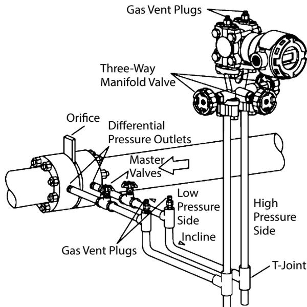
Figure 2-35. Example of Piping for Gas Flow Rate Measurement
