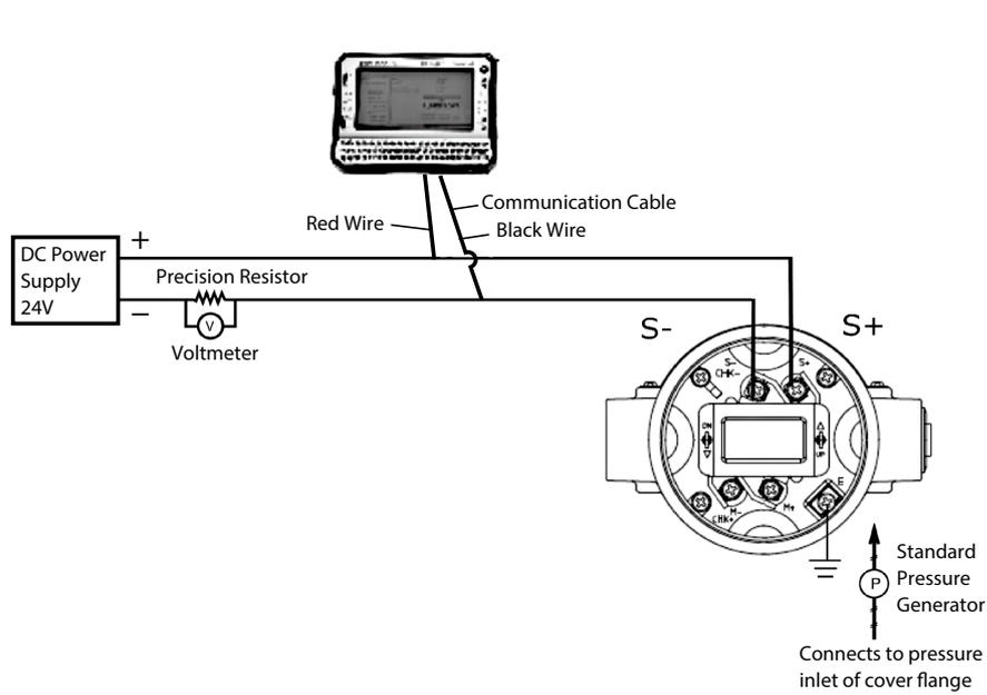
Figure 4-3. Wiring and piping during Calibration
