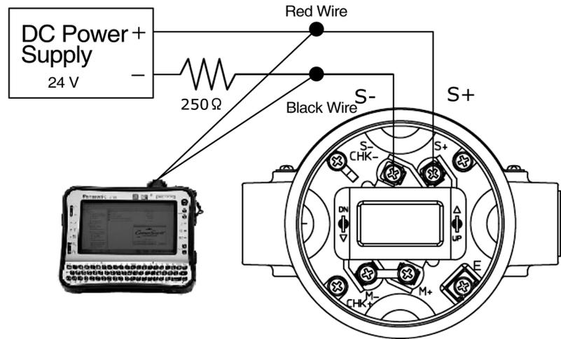
Figure 3-1. Communicator Connection
