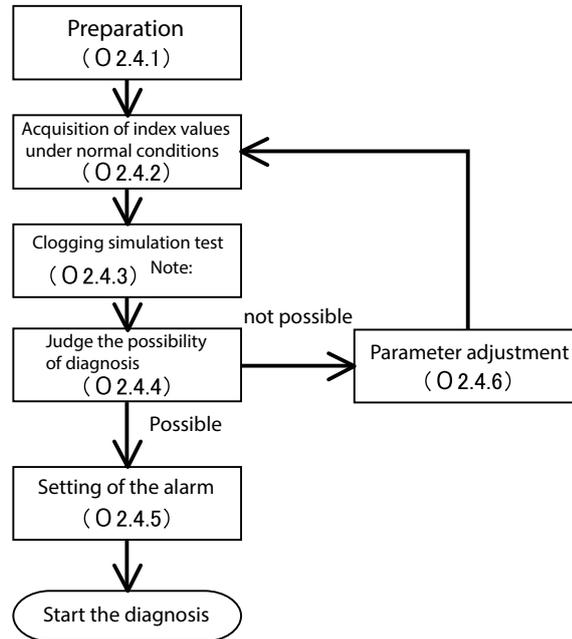
Preparation (see section A2-4-1): Initialize the parameters in preparation for obtaining the index values.
