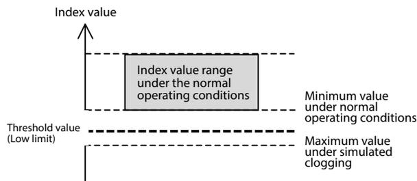
After determining the threshold value, follow the steps below to set the alarm and start the diagnosis.
