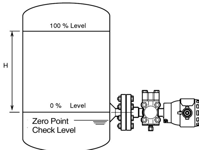
Figure 3-5. Zero Position Determination
