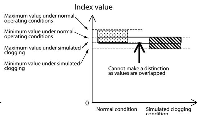
In this case, the index value under normal operating conditions is similar to that with clogging, or the index value is almost the same even when clogging occurs. In either case, it is necessary to examine the cause and to minimize this effect. Use the following guidelines for adjustment.
