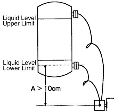
Figure 2-3. Attachment Location for Sealed Tank Level Measurement
