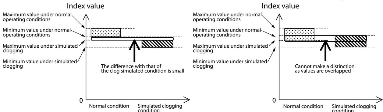
In this case, the index value under normal operating conditions is similar to that with clogging, or the index value is almost the same even when clogging occurs. In either case, it is necessary to examine the cause and to minimize this effect. Use the following guidelines for adjustment.
