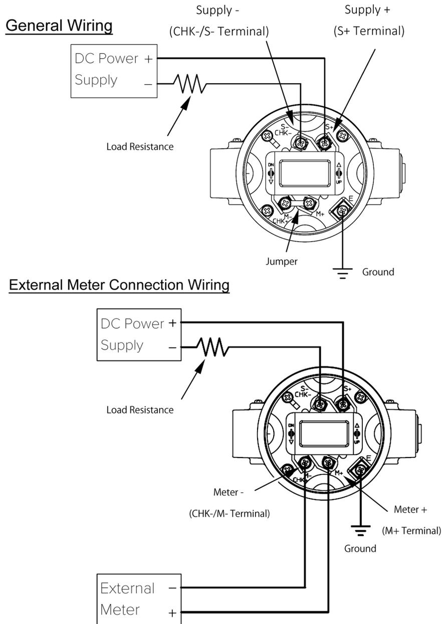
Figure 2-46. Wiring
