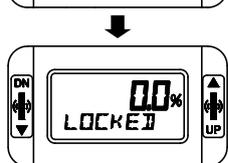
“LOCKED” is displayed for 3 seconds, after which the external adjustment function is disabled.
