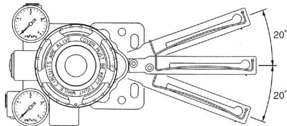
Figure 2-4. Feedback Lever Operating Angle
