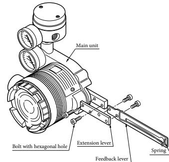
Attachment of Extension Lever and Feedback Lever
