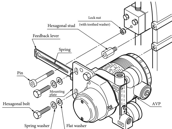
Figure 2-1-1. Mounting the Device on an HA1 Actuator
