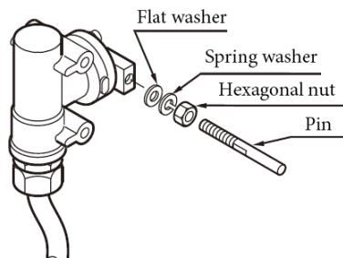
Attachment of Feedback Lever (Pin)
