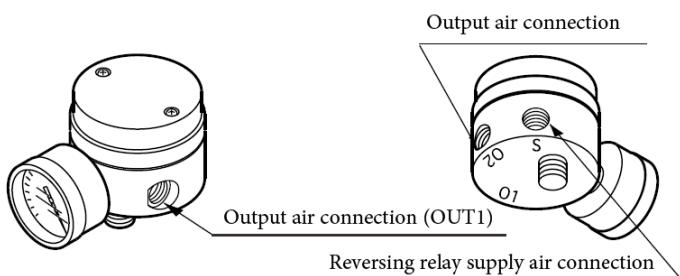
Figure 2-9. Reversing Relay Standalone View
