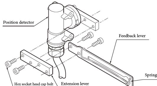
Attachment of Extension Lever and Feedback Lever
