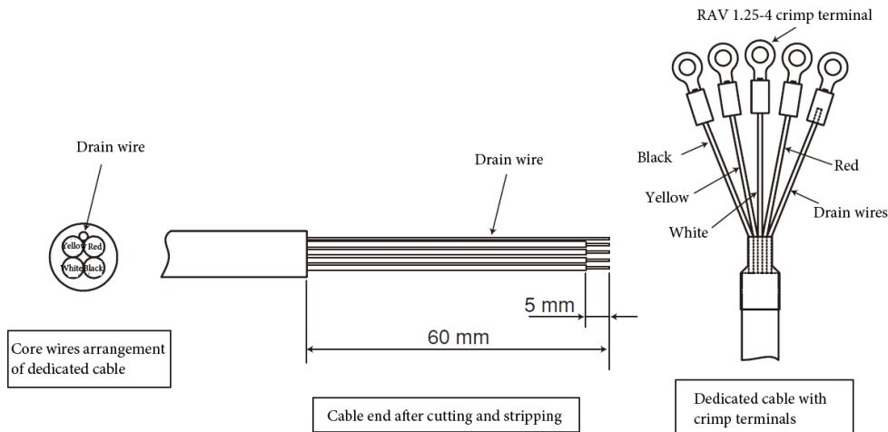
Figure 2-19. Adjusting the Length of the Cable
