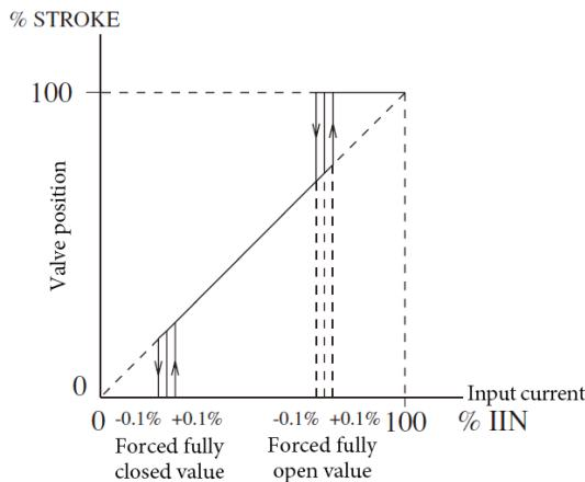
Figure 4-5. Forced Fully Open/Closed Settings
