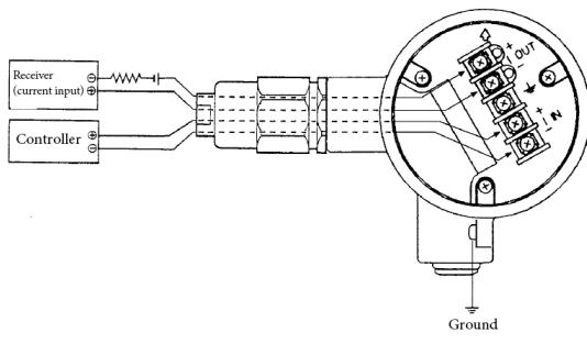
Figure 2-15-1. Wiring for Systems Using a Position Signal
