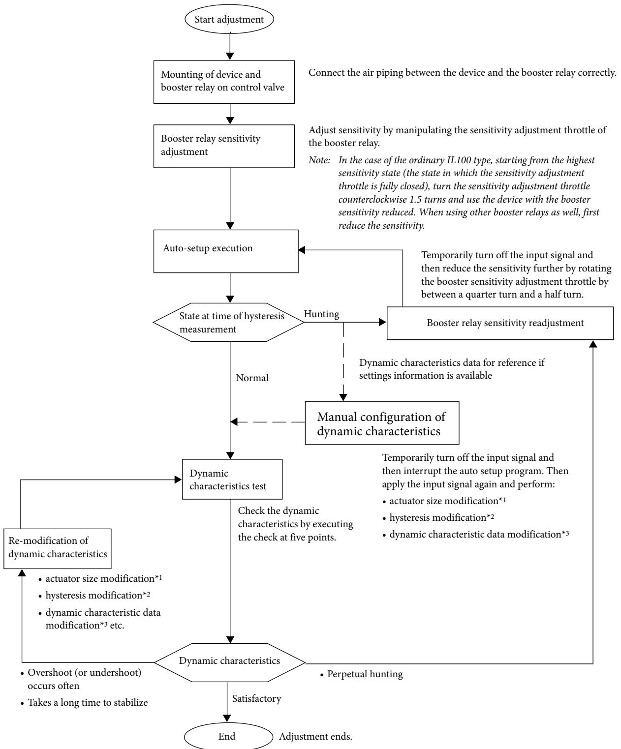
\*1. Change the actuator size parameter such that it becomes progressively smaller: 6 to 5, 5 to 4, ...
