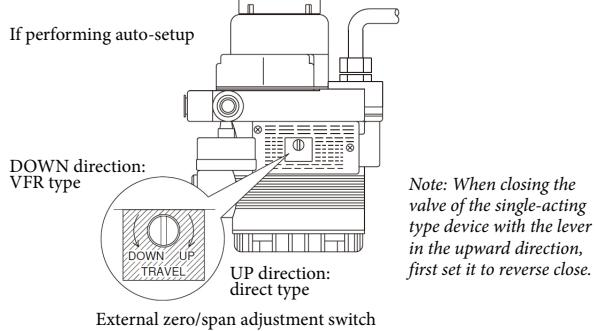
External zero/span adjustment switch
