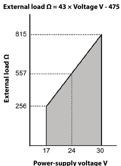
Figure 2-16. Supply Voltage and Load Resistance Characteristics
