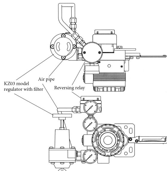
Figure 2-10-2. Air Pipe to Reversing Relay when Model KZ03 Is Installed Integrally
