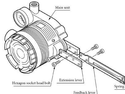
Attachment of Extension Lever and Feedback Lever
