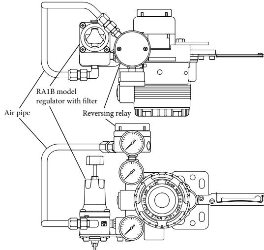
Figure 2-10-1. Air Pipe to Reversing Relay when Model RA1B Is Installed Integrally
