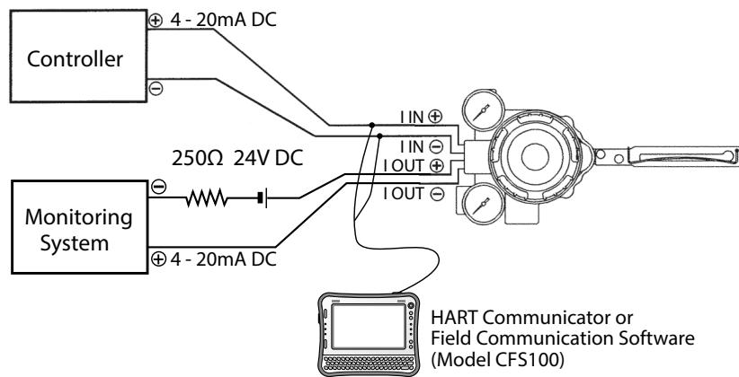
Figure 1-2. Structure of System with Analog Output (Models AVP307 and AVP207)
