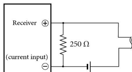
Figure 2-15-3. Wiring if Receiver is Voltage Input Device
