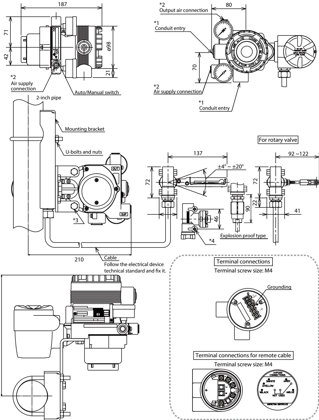
Note 1: Rotary angle should never exceed  $\pm 30^\circ$ .
