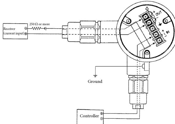
Figure 2-15-2. Wiring for Systems Using a Position Signal
