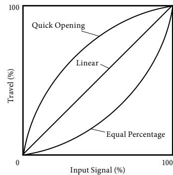
**Figure 1. Input-output characterization**
