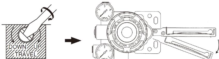
Figure 3-2-2. Adjusting the Lever in the Downward Direction
