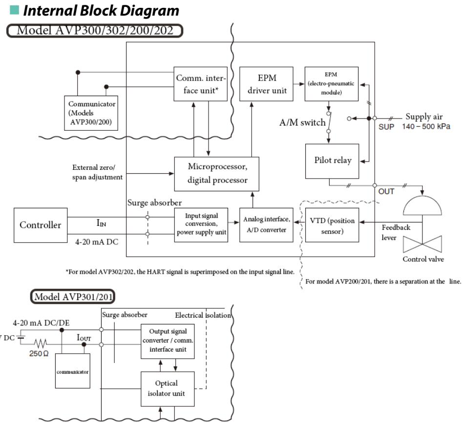
Figure 5-6. Internal Block Diagram
