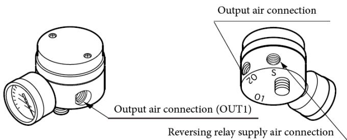
Figure 2-9. Reversing Relay Standalone View
