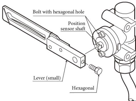
Figure 2-20. Valve Travel Detector
