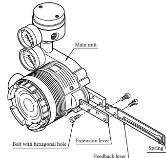
Attachment of Extension Lever and Feedback Lever
