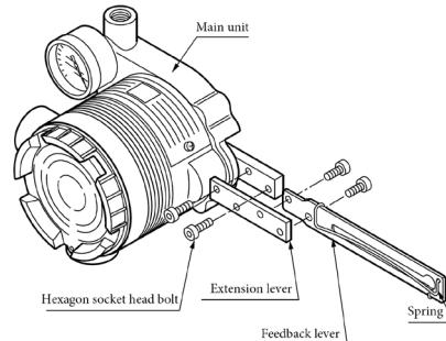
Attachment of Extension Lever and Feedback Lever
