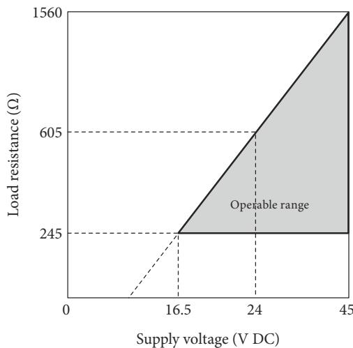
Figure 2-16. Supply Voltage and Load Resistance Characteristics
