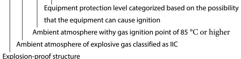
Specifically, the hazardous areas in which the device can be installed are Type 1 areas and Type 2 areas. The device cannot be installed in Type 0 areas.
