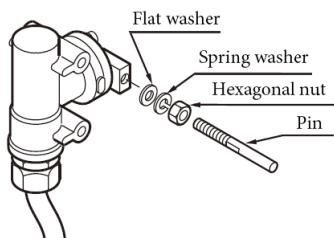
Attachment of feedback lever (pin)
