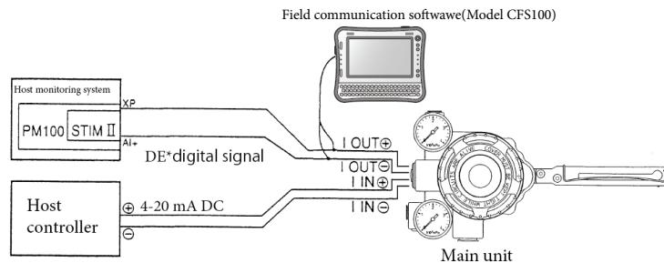
Figure 1-4. Structure of System with Digital Output (Models AVP301 and AVP201)
