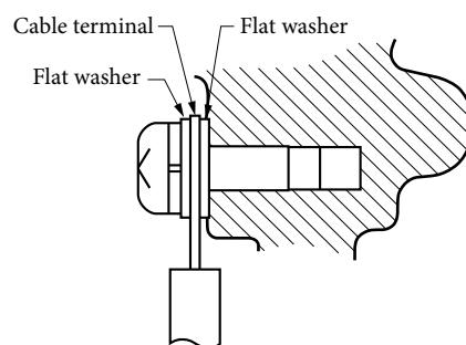
Figure 2-13. Connection to the external ground terminal
