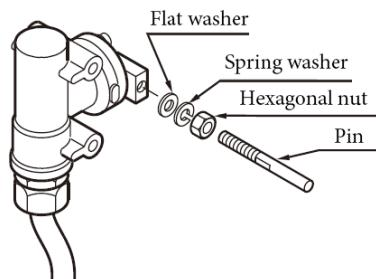
Attachment of Feedback Lever (Pin)
