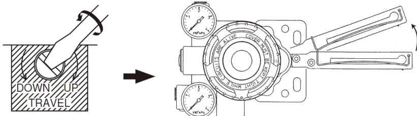
Figure 3-2-1. Adjusting the Lever in the Upward Direction
