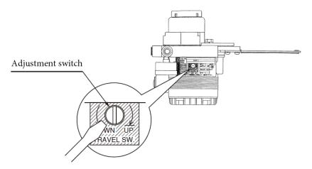
Figure 3-1. External Zero/Span Adjustment Unit Structure
