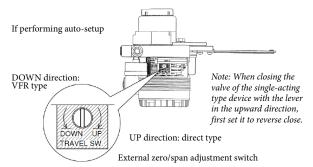
• Auto-setup can be performed with Field Communication Software(Model CFS100) as well.
