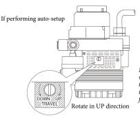
Note: When closing the valve of the single-acting type device with the lever in the upward direction, first set it to reverse close.
