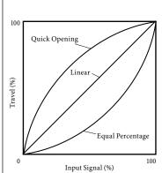
Figure 1. Input-output characterization
