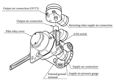
Figure 1-5-2. Body Structure (Rear)
