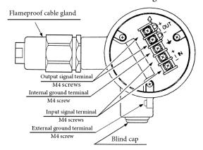
Figure 2-12. Terminal Block of Terminal Box
