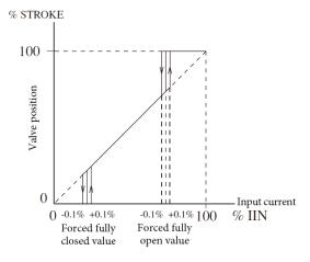
Figure 4-5. Forced Fully Open/Closed Settings
