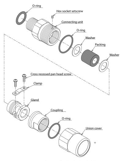
Figure 2-23. Flameproof Cable Gland Exploded View
