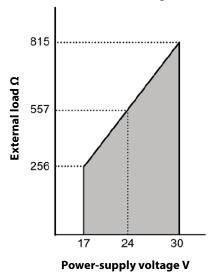
Figure 2-16. Supply Voltage and Load Resistance Characteristics
