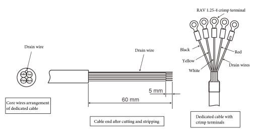
Figure 2-19. Adjusting the Length of the Cable
