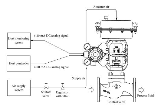
Figure 1-1. Control System Overview Diagram
