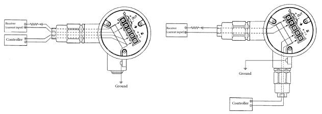
Figure 2-15-1. Wiring for Systems Using a Position Signal (Four-Line Cable)
