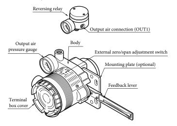
Figure 1-5-1. Body Structure (Front)
