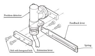
Attachment of Extension Lever and Feedback Lever
