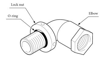
Figure 2-24. Explosion-proof Elbow Structure
