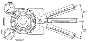
Figure 2-4. Feedback Lever Operating Angle
