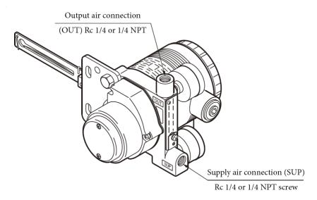
Figure 2-7. Air Piping Connection
