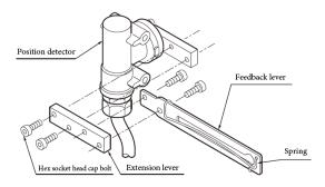
Attachment of Extension Lever and Feedback Lever
