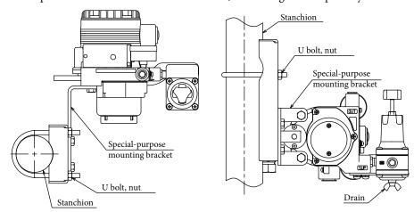
Figure 2-21. Positioner Body Installation
