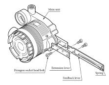
Attachment of Extension Lever and Feedback Lever
