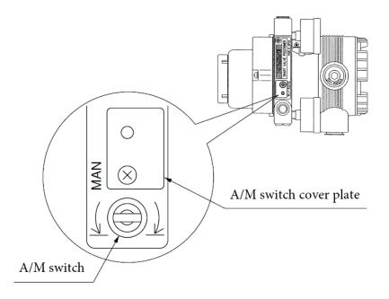
Figure 5-3. A/M Switch Structure
