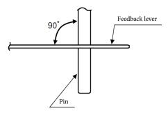
Figure 2-3. Angle between Feedback Lever and Pin
