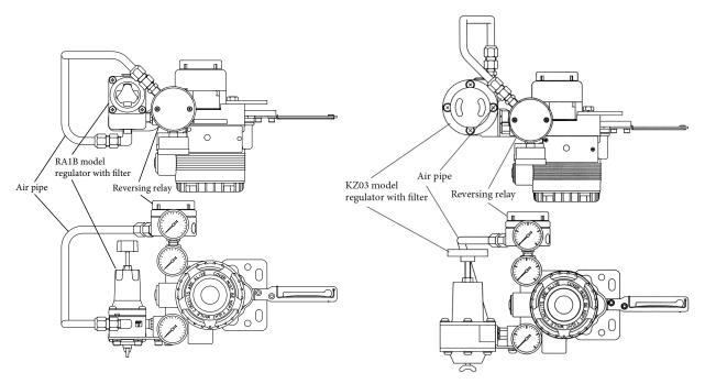
Figure 2-10-1. Air Pipe to Reversing Relay when Model RA1B Is Installed Integrally
