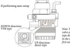
Note: When closing the valve of the single-acting type device with the lever in the upward direction, first set it to reverse close.
