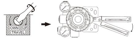
Figure 3-2-2. Adjusting the Lever in the Downward Direction
