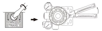
Figure 3-2-1. Adjusting the Lever in the Upward Direction
