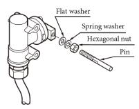
Attachment of Feedback Lever (Pin)
