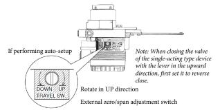
• Auto-setup can be performed with Field Communication Software(Model CFS100) as well.
