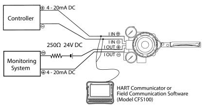
Figure 1-2. Structure of System with Analog Output (Models AVP307 and AVP207)
