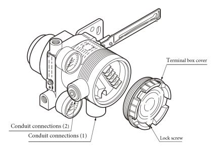
Figure 1-6. Structure of Terminal Box
