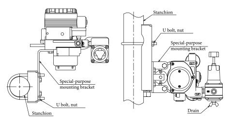
Figure 2-21. Positioner Body Installation
