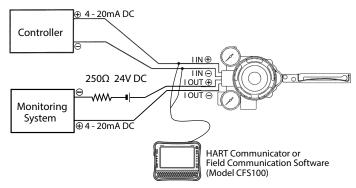
Figure 4-1. Wiring of HART Communication Tool
