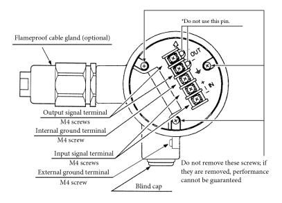
Figure 1-7. Terminal Block of Terminal Box
