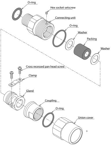
Figure 2-23. Flameproof Cable Gland Exploded View
