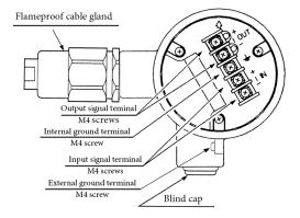
Figure 2-12. Terminal Block of Terminal Box
