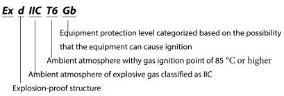
Specifically, the hazardous areas in which the device can be installed are Type 1 areas and Type 2 areas. The device cannot be installed in Type 0 areas.
