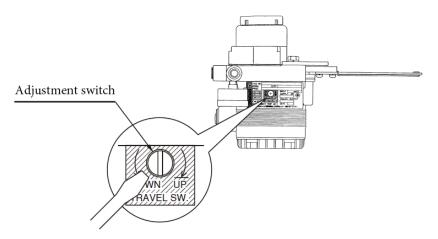
Figure 3-1. External Zero/Span Adjustment Unit Structure
