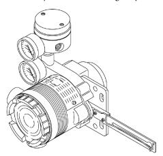
Figure 2-8. Reversing Relay Connection
