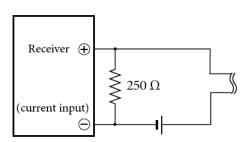
Figure 2-15-3. Wiring if Receiver is Voltage Input Device
