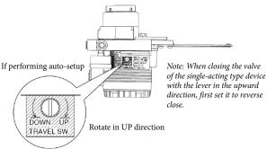
External zero/span adjustment switch
