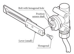
Figure 2-20. Valve Travel Detector
