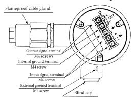
Figure 2-12. Terminal Block of Terminal Box
