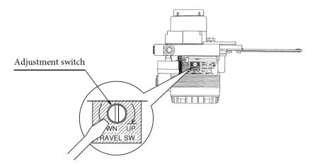
Figure 3-1. External Zero/Span Adjustment Unit Structure
