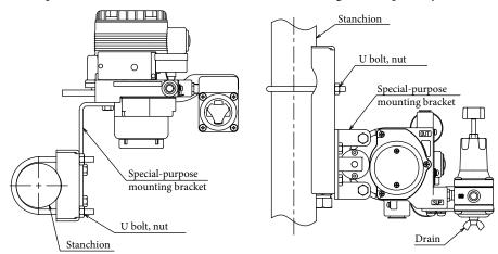
Figure 2-21. Positioner Body Installation
