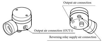
Figure 2-9. Reversing Relay Standalone View
