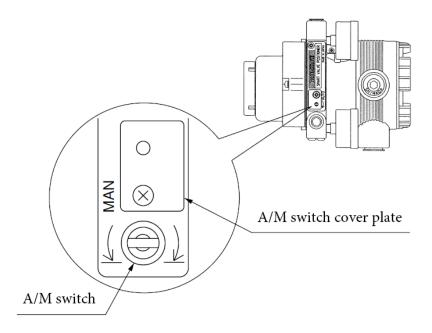
Figure 5-5. A/M Switch Structure
