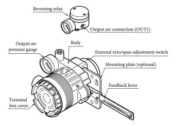
Figure 1-5-1. Body Structure (Front)
