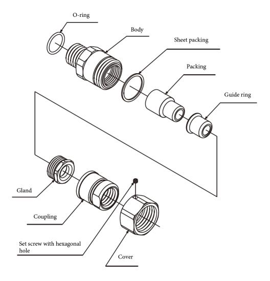
Figure 2-25. Flameproof Cable Gland Exploded View
