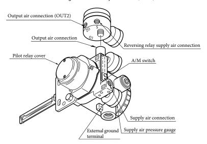
Figure 1-5-2. Body Structure (Rear)
