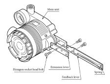
Attachment of Extension Lever and Feedback Lever
