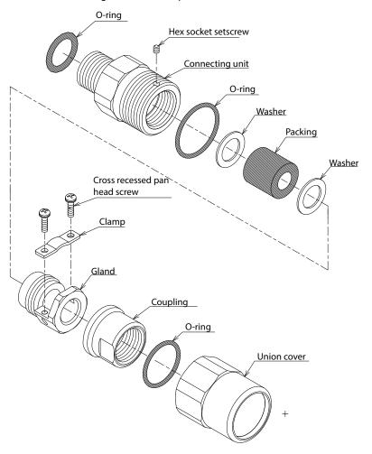
Figure 2-23. Flameproof Cable Gland Exploded View
