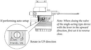
External zero/span adjustment switch
