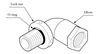
Figure 2-26. Explosion-proof Elbow Structure
