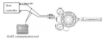
Figure 4-1. Wiring of HART Communication Tool (Models AVP302/202)
