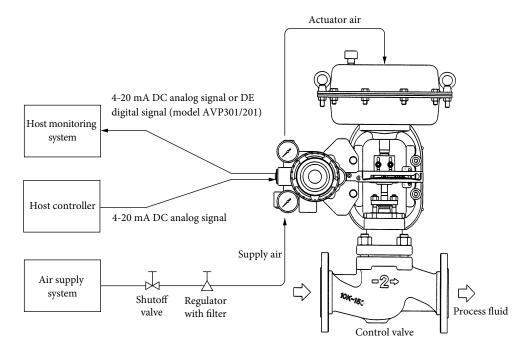
Figure 1-1. Control System Overview Diagram
