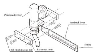
Attachment of Extension Lever and Feedback Lever
