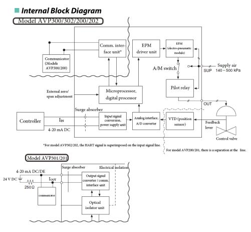
Figure 5-6. Internal Block Diagram
