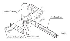
Attachment of Extension Lever and Feedback Lever
