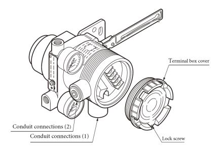
Figure 1-6. Structure of Terminal Box
