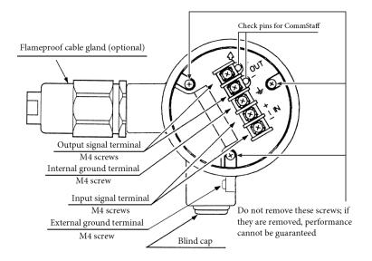
Figure 1-7. Terminal Block of Terminal Box
