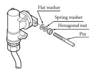
Attachment of feedback lever (pin)
