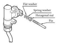
Attachment of Feedback Lever (Pin)
