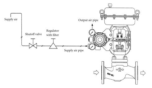
Figure 2-6. Air Supply System
