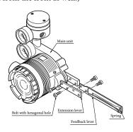
Attachment of Extension Lever and Feedback Lever
