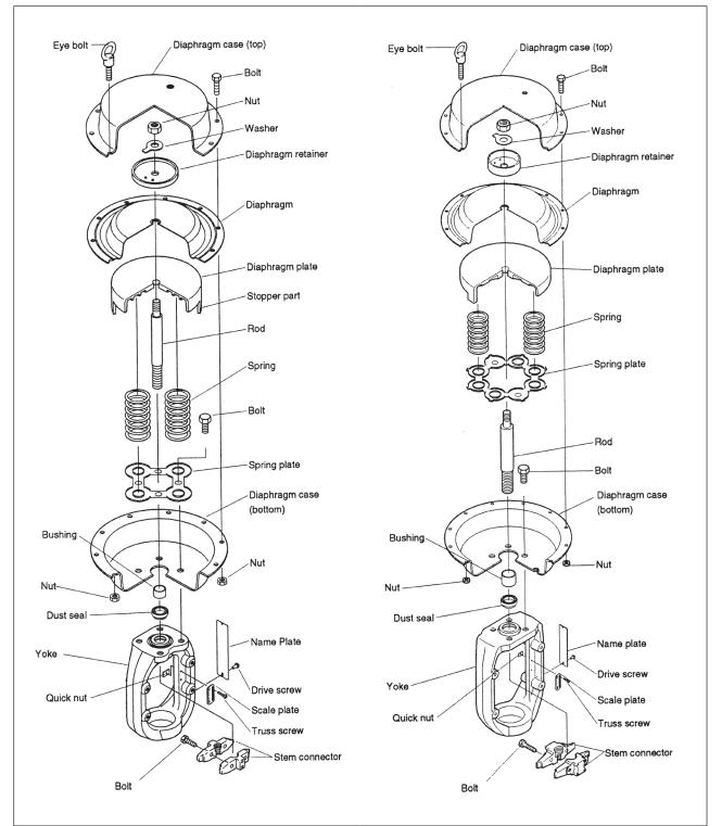
Fig. 4-5. Direct Action model (Model PSA1D, PSA2D)
