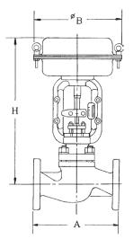
Fig. A-1. face-to-face dimension and overall dimensions
