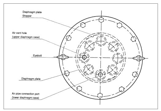
Fig. 4-15. Reverse Action models:Model PSA3R Actuator
