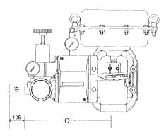
Fig. A-4. model HEP positioner mounted \*When applying a presureproof packing, add 105 mm
