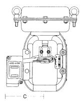
Fig. A-2. model VPE positioner mounted
