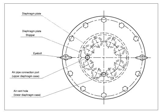
Fig. 4-11. Direct Action models: Model PSA3D Actuator
