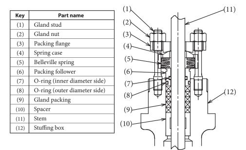
Fig. 6-1. Structural drawing of Azbil low emission gland packing
