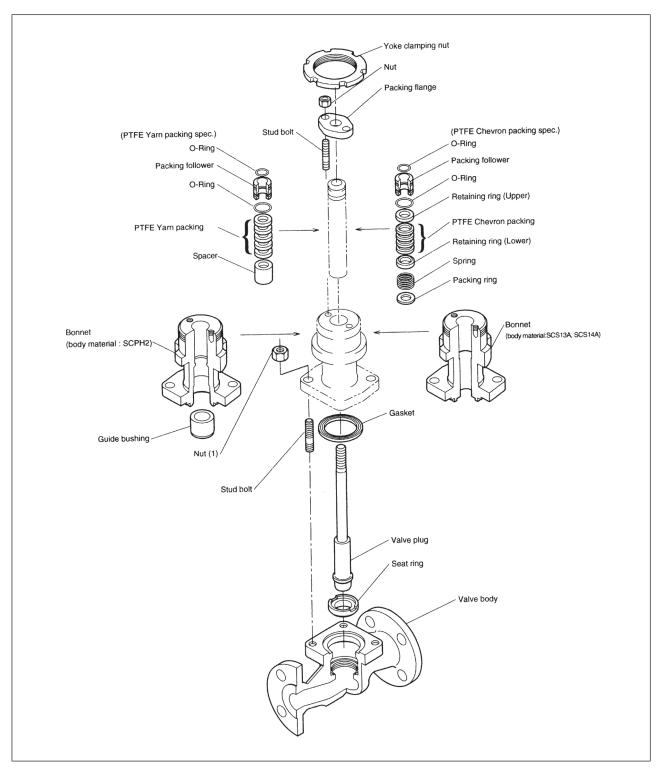
Fig. 4-2. Model AGVB Control Valve (Available body sizes: 1/2 inches, 3/4 inches, 1 inch)
