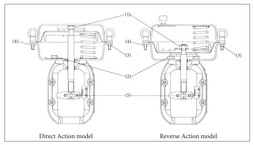
Fig. 4-17. Bolts and Nuts of Actuator
