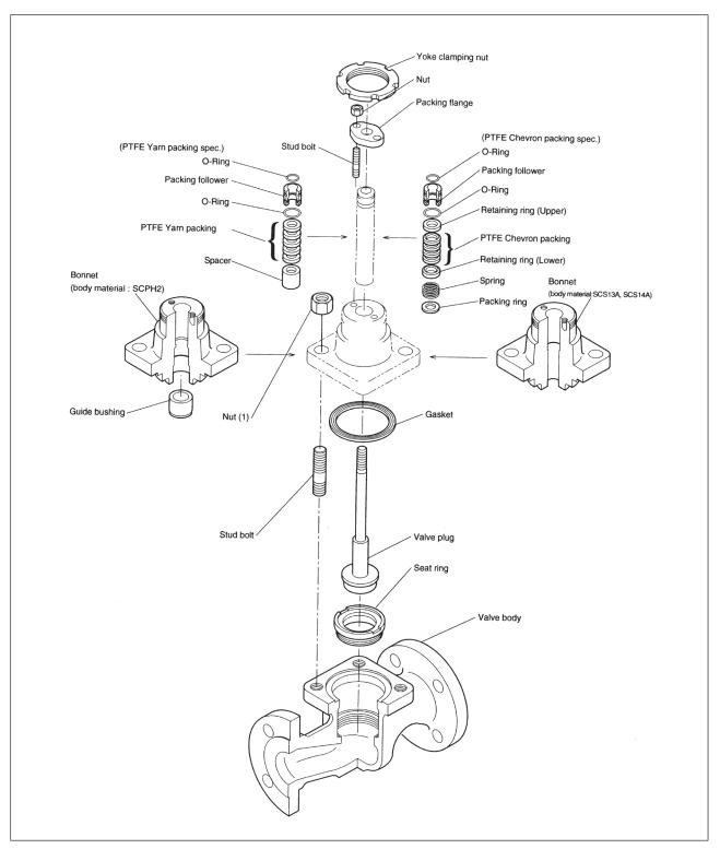
Fig. 4-3. Model AGVB Control Valve (Available body sizes: 1-1/2 inches, 2 inches)
