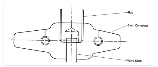
Fig. 5-1. Adjustment for Direct or Reverse Action models
