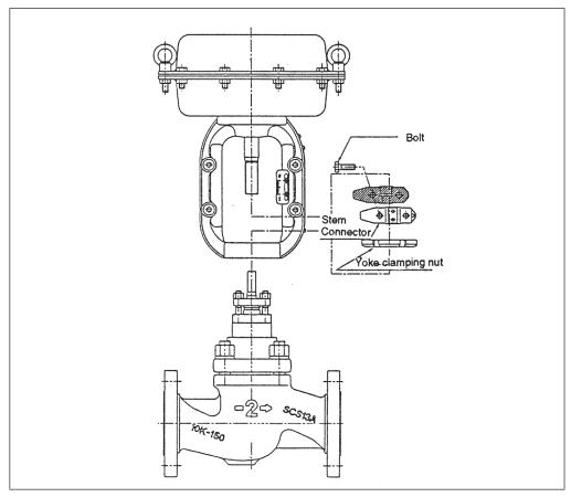
Fig. 4-1. Disassembling the actuator
