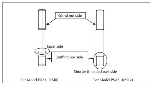
Fig. 6-2. Direction of the gland studs
