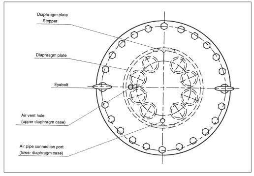
Fig. 4-16. Reverse Action models:Model PSA4R Actuator
