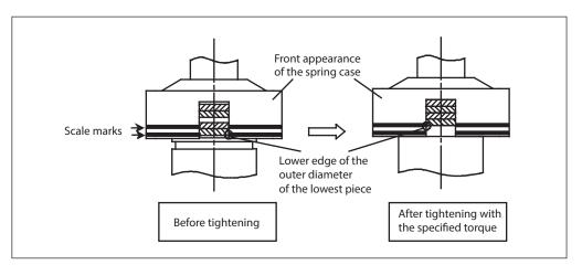
Fig. 6-5. Loading conditions of the Belleville springs
