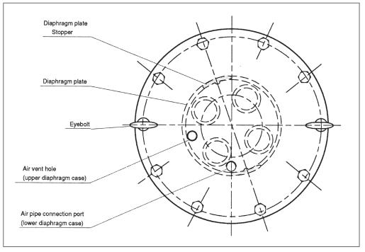
Fig. 4-14. Reverse Action models: Model PSA2R Actuator
