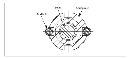
Fig. 6-4. Installation of the spring case Top view
