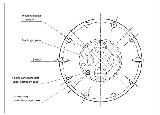
Fig. 4-10. Direct Action models: Model PSA2D Actuator
