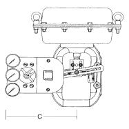
Fig. A-3. model HTP positioner mounted
