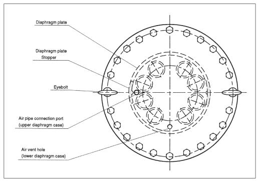
Fig. 4-12. Direct Action models: Model PSA4D Actuator
