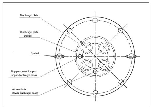
Fig. 4-9. Direct Action models: Model PSA1D Actuator
