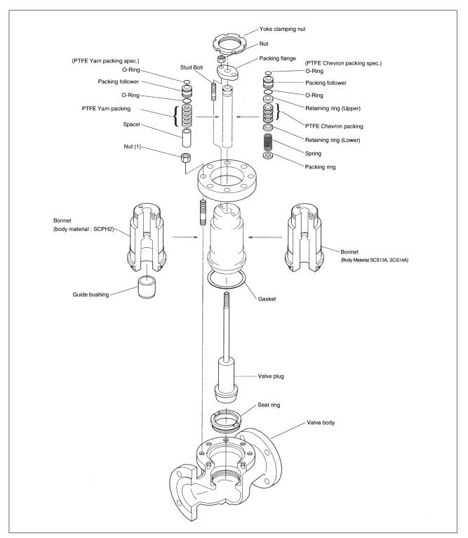
Fig. 4-4. Model AGVB Control Valve (Available body sizes: 2-1/2 inches, 3 inches, 4 inches)
